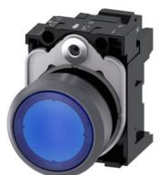
Indicator light, in illuminated pushbutton design, 22 mm, round, plastic with metal front ring, blue, with holder, LED module, with integrated LED 24 V AC/DC, Spring-type terminal
