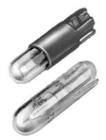
incandescent lamp, clear, rated voltage 24 V AC/DC, 1.0 W Wedge base W2 x 4.6 d,
