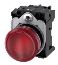
Indicator lights, 22 mm, round, metal, shiny, red, lens, smooth, with holder, LED module with integrated LED 24 V AC/DC, screw terminal, with laser labeling, lower case
