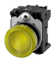
Indicator lights, 22 mm, round, metal, shiny, yellow, lens, smooth, with holder, LED module with integrated LED 110 V AC, screw terminal, Z=20-unit packaging
