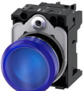
Indicator lights, 22 mm, round, metal, shiny, blue, lens, smooth, with holder, LED module with integrated LED 110 V AC, screw terminal, with laser labeling, symbol number according to, ISO 7000 or IEC 60417
