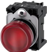
Indicator lights, 22 mm, round, metal, shiny, red, lens, smooth, with holder, LED module with integrated LED 110 V AC, screw terminal, with laser labeling, symbol number according to, ISO 7000 or IEC 60417
