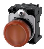
Indicator lights, 22 mm, round, plastic, amber, lens, smooth, with holder, LED module with integrated LED 110 V AC, screw terminal
