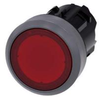
Indicator light in illuminated pushbutton design, 22 mm, round, plastic with metal front ring, red, with laser labeling, upper case and lower case, always upper case at the beginning of the word
