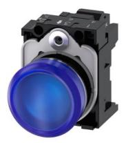
Indicator lights, 22 mm, round, metal, shiny, blue, lens, smooth, with holder, LED module with integrated LED 24 V AC/DC, spring-type terminal, with laser labeling, lower case
