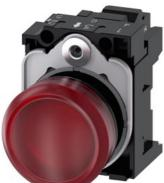
Indicator lights, 22 mm, round, plastic, red, lens, smooth, with holder, LED module, with integrated LED 24 V AC/DC, Spring-type terminal
