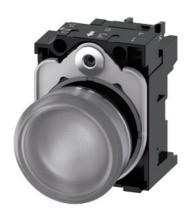
Indicator lights, 22 mm, round, metal, shiny, clear, lens, smooth, with holder, LED module with integrated LED 24 V AC/DC, screw terminal, with laser labeling, symbol number according to, ISO 7000 or IEC 60417
