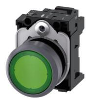
Indicator light, in illuminated pushbutton design, 22 mm, round, plastic with metal front ring, green, with holder, LED module, with integrated LED 24 V AC/DC, Spring-type terminal
