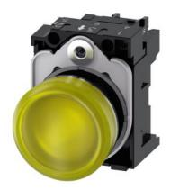
Indicator lights, 22 mm, round, metal, shiny, yellow, lens, smooth, with holder, LED module with integrated LED 24 V AC/DC, screw terminal, with laser labeling, inscription or symbol Customer-specific selection with SIRIUS ACT configurator (CIN)
