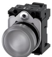
Indicator lights, 22 mm, round, metal, shiny, clear, lens, smooth, with holder, LED module with integrated LED 24 V AC/DC, spring-type terminal, with laser labeling, upper case
