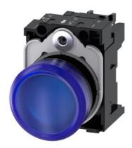
Indicator lights, 22 mm, round, plastic, blue, lens, smooth, with holder, LED module, with integrated LED 24 V AC/DC, screw terminal, with laser labeling, upper case and lower case, always upper case at the beginning of the word
