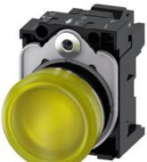
Indicator lights, 22 mm, round, Metal, shiny, yellow, lens, smooth, with holder, LED module with integrated LED 230 V AC, spring-type terminal, with laser labeling, upper case
