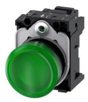
Indicator lights, 22 mm, round, plastic, green, lens, smooth, with holder, LED module, with integrated LED 24 V AC/DC, spring-type terminal, Z=20-unit packaging
