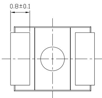
For reflow soldering (propose)
