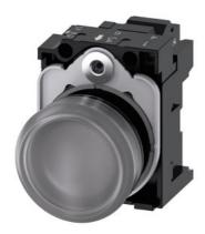
Indicator lights, 22 mm, round, plastic, clear, lens, smooth, with holder, LED module, with integrated LED 230 V AC, spring-type terminal, with laser labeling, upper case and lower case, always upper case at the beginning of the word
