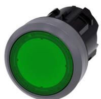
Indicator light in illuminated pushbutton design, 22 mm, round, plastic with metal front ring, green, with laser labeling, symbol number according to, ISO 7000 or IEC 60417
