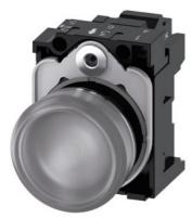
Indicator lights, 22 mm, round, metal, shiny, clear, lens, smooth, with holder, LED module with integrated LED 110 V AC, Spring-type terminal
