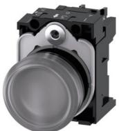
Indicator lights, 22 mm, round, plastic, clear, lens, smooth, with holder, LED module, with integrated LED 230 V AC, screw terminal, with laser labeling, upper case and lower case, always upper case at the beginning of the word
