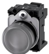
Indicator lights, 22 mm, round, plastic, clear, lens, smooth, with holder, LED module, with integrated LED 110 V AC, spring-type terminal, with laser labeling, upper case and lower case, always upper case at the beginning of the word
