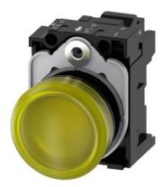
Indicator lights, 22 mm, round, plastic, yellow, lens, smooth, with holder, LED module with integrated LED 110 V AC, spring-type terminal, with laser labeling, upper case and lower case, always upper case at the beginning of the word
