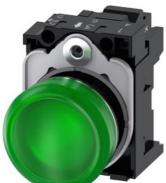
Indicator lights, 22 mm, round, metal, shiny, green, lens, smooth, with holder, LED module with integrated LED 24 V AC/DC, spring-type terminal, with laser labeling, upper case and lower case, always upper case at the beginning of the word
