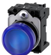
Indicator lights, 22 mm, round, metal, shiny, blue, lens, smooth, with holder, LED module with integrated LED 24 V AC/DC, screw terminal, with laser labeling, lower case
