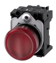
Indicator lights, 22 mm, round, plastic, red, lens, smooth, with holder, LED module, with integrated LED 230 V AC, screw terminal, with laser labeling, lower case
