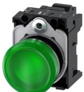
Indicator lights, 22 mm, round, metal, shiny, green, lens, smooth, with holder, LED module with integrated LED 110 V AC, spring-type terminal, Z=20-unit packaging
