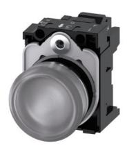
Indicator lights, 22 mm, round, metal, shiny, clear, lens, smooth, with holder, LED module with integrated LED 24 V AC/DC, spring-type terminal, with laser labeling, symbol number according to, ISO 7000 or IEC 60417
