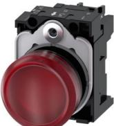
Indicator lights, 22 mm, round, plastic, red, lens, smooth, with holder, LED module with integrated LED 110 V AC, screw terminal, with laser labeling, upper case
