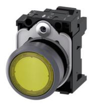
Indicator light, in illuminated pushbutton design, 22 mm, round, plastic with metal front ring, yellow, with holder, LED module, with integrated LED 24 V AC/DC, Spring-type terminal
