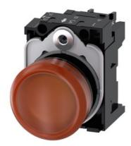
Indicator lights, 22 mm, round, plastic, amber, lens, smooth, with holder, LED module, with integrated LED 230 V AC, screw terminal, with laser labeling, upper case and lower case, always upper case at the beginning of the word
