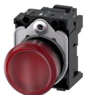
Indicator lights, 22 mm, round, plastic, red, lens, smooth, with holder, LED module, with integrated LED 24 V AC/DC, spring-type terminal, with laser labeling, lower case
