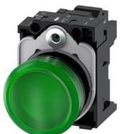
Indicator lights, 22 mm, round, plastic, green, lens, smooth, with holder, LED module, with integrated LED 24 V AC/DC, spring-type terminal, with laser labeling, symbol number according to, ISO 7000 or IEC 60417
