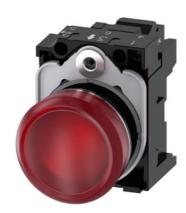
Indicator lights, 22 mm, round, Metal, shiny, red, lens, smooth, with holder, LED module with integrated LED 230 V AC, spring-type terminal, with laser labeling, upper case and lower case, always upper case at the beginning of the word
