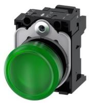
Indicator lights, 22 mm, round, plastic, green, lens, smooth, with holder, LED module, with integrated LED 230 V AC, spring-type terminal, with laser labeling, upper case
