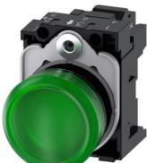
Indicator lights, 22 mm, round, plastic, green, lens, smooth, with holder, LED module, with integrated LED 24 V AC/DC, Spring-type terminal
