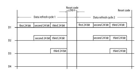
Note: The data of D1 is sent by MCU, and D2,D3,D4 through pixel internal reshaping amplification to transmit.
