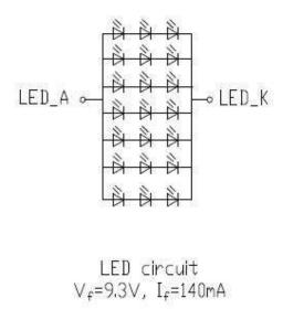
Figure 4.1 LED connection of backlight
