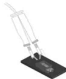
Fig2. Repairing using a double-head soldering iron
