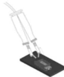
Fig2. Repairing using a double-head soldering iron
