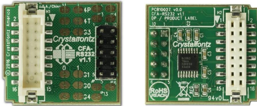
Figure 14. CFA-RS232 Top (left) and Bottom View of Connectors
