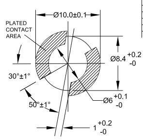
PC BOARD PUNCH PATTERN (NO TREATMENT, SUCH AS APPLICATION OF FLUX, SHALL BE DONE.)
