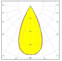
Dimensions: 1140.0 mm x 40.0 mm Height: 20.20 mm ~50° wide beam with tighter cutoff. Variant with 7X1 lenses.
