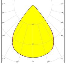
Dimensions: 1140.0 mm x 40.0 mm Height: 20.20 mm ~80° wide beam. Variant with diffused 4X1 lenses.
