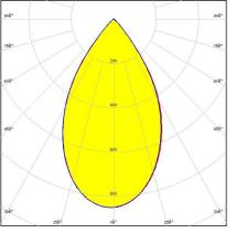
Dimensions: 1140.0 mm x 40.0 mm Height: 20.20 mm ~50° wide beam. Variant with diffused 4X1 lenses.
