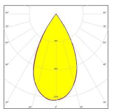
Dimensions: 1140.0 mm x 40.0 mm Height: 20.20 mm ~50° wide beam. Variant with 4X1 lenses.
