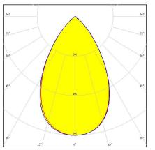
Dimensions: 1140.0 mm x 40.0 mm Height: 20.20 mm ~50° wide beam with tighter cutoff.
