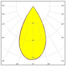
Dimensions: 1140.0 mm x 40.0 mm Height: 20.20 mm ~50° wide beam. Variant with 7X1 lenses.
