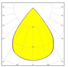
Dimensions: 1140.0 mm x 40.0 mm Height: 20.20 mm ~80° wide beam. Variant with diffused 7X1 lenses.
