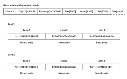
In case 2, while lamp2 is under sleep mode, in the following data transfer process, the state of lamp 2 will be not changed as long as the 32 bits data for lamp 2 is received with data of Flag[2:0] DIMMING[4:0] being 8h"A0". It means lamp2 will keep in sleep mode as well. In the situation, lamp2 can pass through the remaining data to lamp 3 (32bits) to change the display data of lamp 3. In other words, the sleeping chip is able to pass the data to the next chips.
