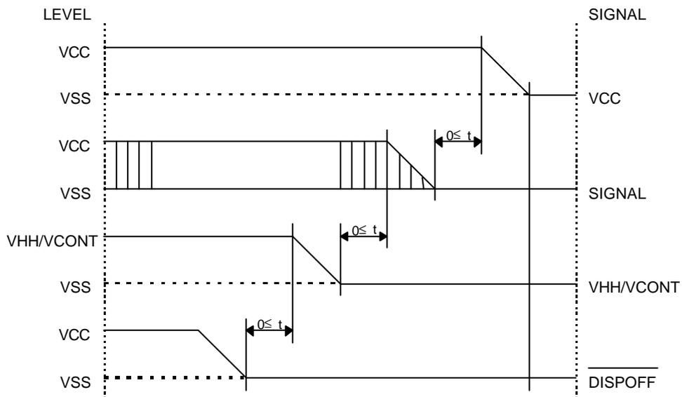
Please maintain the above sequence when turning on and off the power supply of the module.
