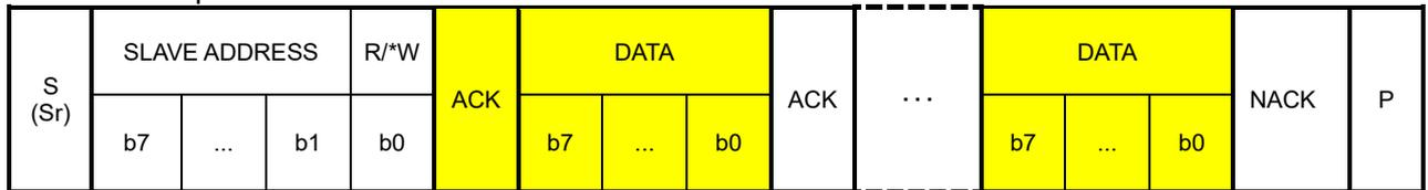
Host (master) is transmitter, display module (slave) is receiver
