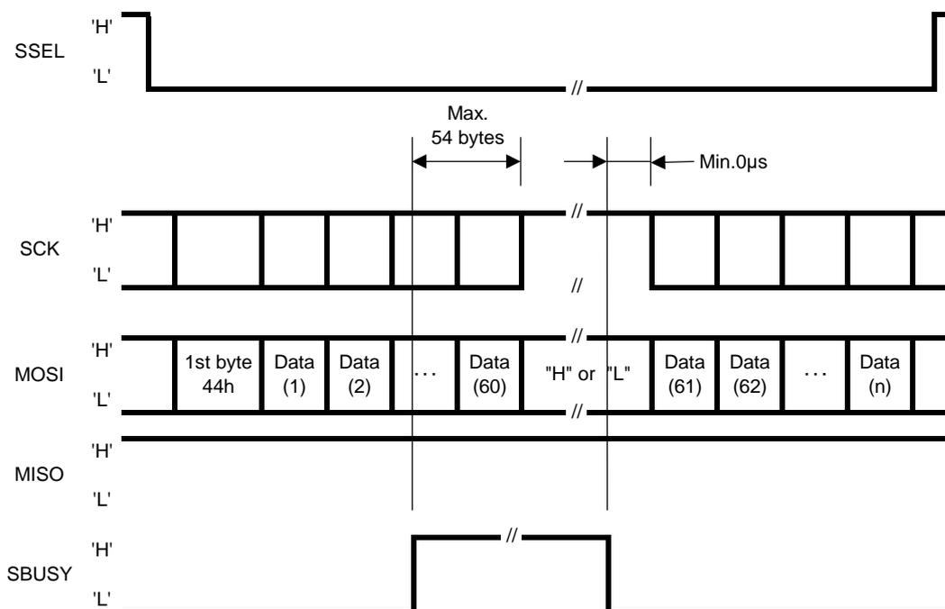
When confirming the SBUSY signal by status read, make one command sequence 54 bytes or less.
