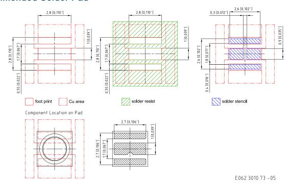
For superior solder joint connectivity results we recommend soldering under standard nitrogen atmosphere. Further information can be found in our Application Note: "Handling and Processing Details for Ceramic LEDs".
