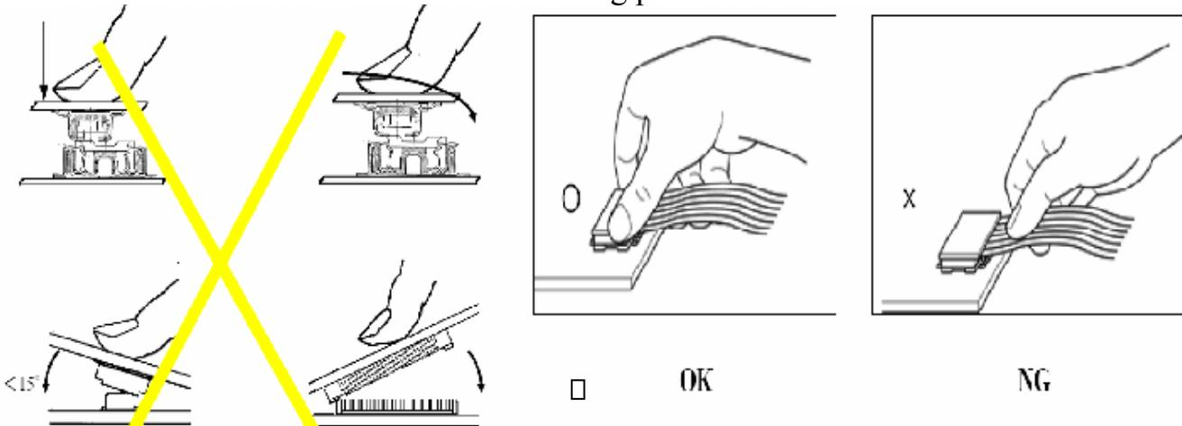
**Precaution for soldering to the LCM**
