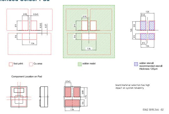
For superior solder joint connectivity results we recommend soldering under standard nitrogen atmosphere. Package not suitable for ultra sonic cleaning. To ensure a high solder joint reliability and to minimize the risk of solder joint cracks, the customer is responsible to evaluate the combination of PCB board and solder paste material for his application.
